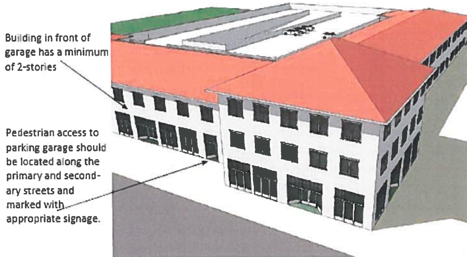
Figure 7.02.03.G: Building Design, Building in Front of Parking Garage
