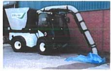
Features include a 1.5 y<sup>3</sup> collection container capacity. The CityVac attachment is designed to operate between 1250 - 1500 engine RPM, reducing fuel consumption and noise pollution. A Low noise fan and heavy-duty, microbe-resistant vacuum hose make if ideal for use even in close proximity of other ground staff. The CityVac concept originated from North American demand where airport customers wanted a vacuum unit that can also be multipurpose and include off road capability.
