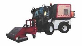
built-in high-pressure spray nozzles for runway surface cleaning. The high temperature steam coupled with the high-pressure spray nozzles allow for superior cleaning without the use of any cleaning agents or chemicals. The front spray bar system is 47" wide and depending on the model comes with 158 gal, 290 gal, 396 gal capacities.
